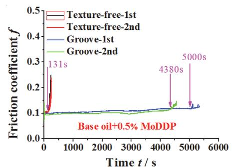
Fig. 2. Effective lubrication time (groove)
