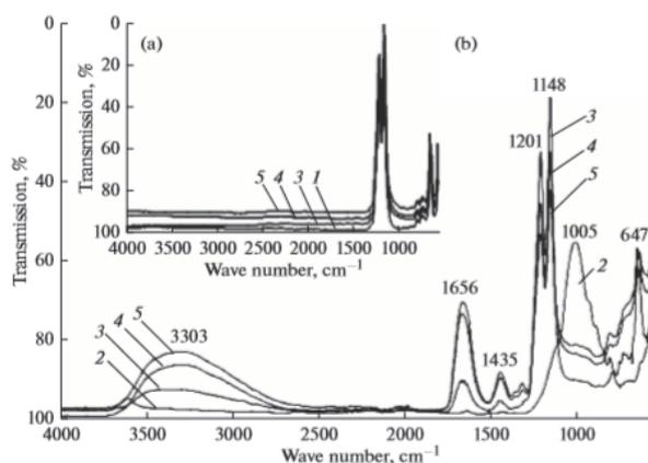
Figure. Typical IR spectra of PTFE composites before (a) and after friction (b)
