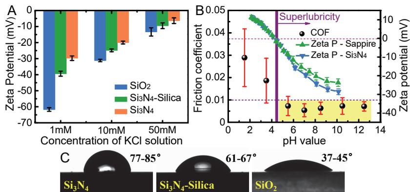
Fig. 3. Effect of the silica layer on the surface potential of Si<sub>3</sub>N<sub>4</sub>
