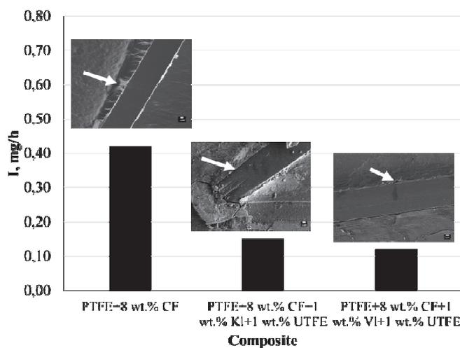
Figure. Results of wear rate and worn surface of PTFE and PCMs
