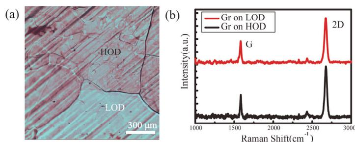
Fig. 1. (a) Optical image of the substrates. (b) The Raman spectra of the graphene layers on substrates
