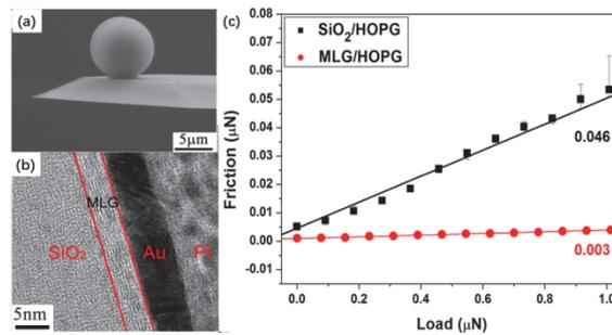
Fig. 5. (a) SEM side view of the graphene-coated microsphere probe. (b) Pt and Au films are deposited as the protective film during TEM sample preparation of focused ion beam process. (c) Friction force as a function of the applied normal load for SiO<sub>2</sub> microsphere sliding against HOPG and MLG-coated SiO<sub>2</sub> microsphere against HOPG respectively [12]
