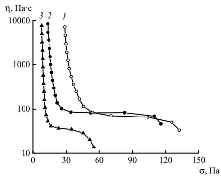
Figure. Flow curves of lubricants at 25 °C based on DOS (1), NB-5750 (2) and NB-7300 (3) containing 10% of the mass of the dodecylamine-based thickener
