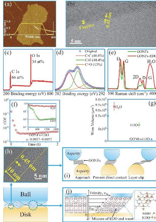
Fig. 4. Characterization of GONFs: (a) atomic force microscopy image; (b) high-resolution transmission electron microscopy (HRTEM) image; (c, d) XPS spectra; (e) Raman spectra. (f, g) Friction and wear testing results for GONFs-EDO. (h) HRTEM image of the cross-sectional area of the worn surface. (i, j) Proposed superlubricity and anti-wear mechanism of GONFs-EDO [9]
