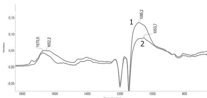
Figure. ATR FTIR subtraction spectra of the friction surfaces of PTFE/SiO<sub>2</sub> (1) and PTFE-A/SiO<sub>2</sub> (2) nanocomposites after friction on 40X steel
