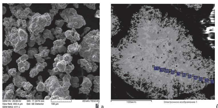
Figure. The new borated powder from the dispersed metal wastes: a – morphology; b – the structure of particles
