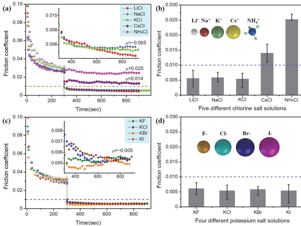
Fig. 1. Friction coefficients under lubrication of 50 mM chloride/potassium salt solutions
