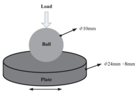
Fig. 1. Schematic of test rig
