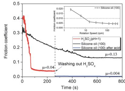
Fig. 3. Friction coefficient of silicone oil and that after running-in process with  $H_2SO_4$  [8]
