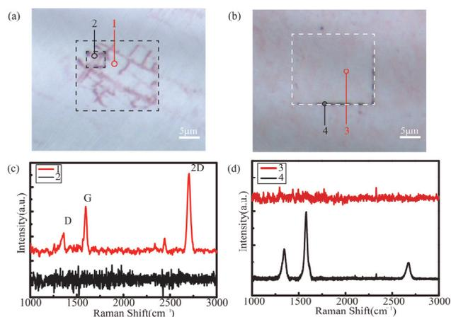
Fig. 3. Optical images of the worn area, a for LOD and b for HOD. Raman spectra obtained in a (c) and b (d)
