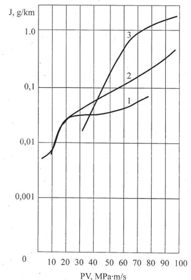
Figure. Dependence of wear for different specific load: 1 – 2.9 MPa; 2 – 7.6 MPa; 3 – 10.7 MPa
