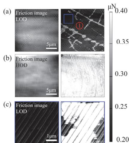
Fig. 2. Friction force images at the same location on (a) LOD and (b) HOD substrates, the normal force was 0.148  $\mu\text{N}$  and 1.48  $\mu\text{N}$  respectively. (c) Friction force images measured within the blue square area in fig. 2a, the normal force was 1.776  $\mu\text{N}$  and 3.108  $\mu\text{N}$  respectively
