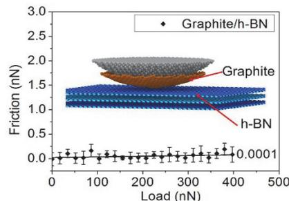
Fig. 6. Friction coefficient between graphite and h-BN [13]
