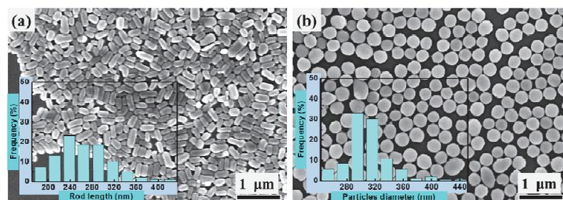
Figure. SEM micrographs of the PTFE latices (a) and PTFE@PMMA (1.5)
